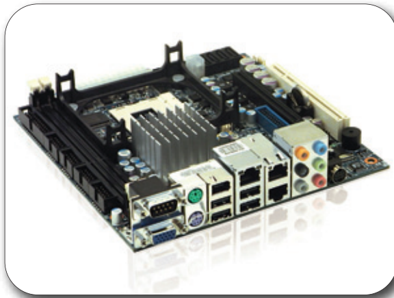
Figure 1. The Kontron KTGM45 embedded motherboard in Mini-ITX, Flex-ATX and ATX form factor offers high reliability, 7 year long-term availability and integrated Intel AMT 4.0.
